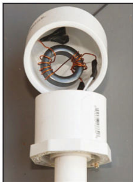
Photo A. Impedance matching toroid in top end of PVC barbell. The first two turns are bifilar wound. The white wire is the coax center conductor connected to the 2-turn primary. Next to it, the primary and secondary wires are connected to the coax braid. Both connections are covered with heat shrink tubing. Cable ties may be added to stabilize wires on the toroid.
