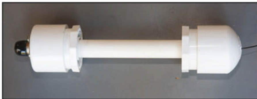
Photo C. Assembled barbell containing impedance-matching toroid at right and common mode choke toroid at left. Total length is 9-1/2 inches, excluding the SO-239 coax connector. The spacing between the top and bottom reducer bushings is 4-1/2 inches. Separating the toroids by 7 inches is a key dimension.
