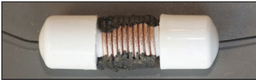
Photo E. Trap showing end caps secured with PVC cement.
