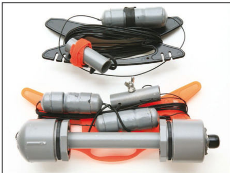
Photo G. Completed EFHW trap antenna (18 oz) with 40-meter extension (4 oz) on SOTAbeam windsors.
